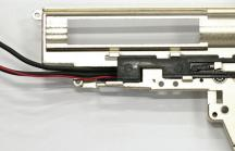
**6.** In the place of the original switch group fix the Sensor Unit by screwing back the screw that was used for the original switch assembly.
