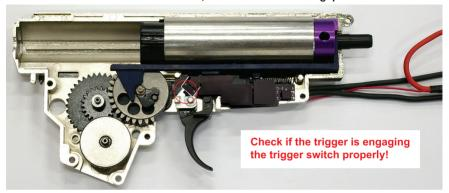
WARNING! Do NOT reinstall the anti-reversal latch! You do not need it anymore. \*Anti-reversal latch may be reinstalled only if you use a low power magnets motor.
