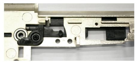
**5.** Separate the ECU and the Mosfet of the ASCU. Pass the wires through the opening in the gearbox shell as shown on the picture.
