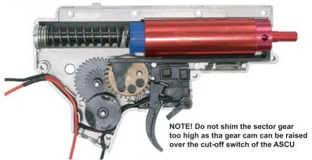
**NOTE:** If you are using a quality high torque motor with strong magnets, you do not need to reinstall the Anti-Reversal Latch (ARL).
