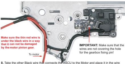
**8.** Take the other Black wire that connects the ASCU to the Motor and place it in the wire channel of the gearbox shell as shown on the picture.
